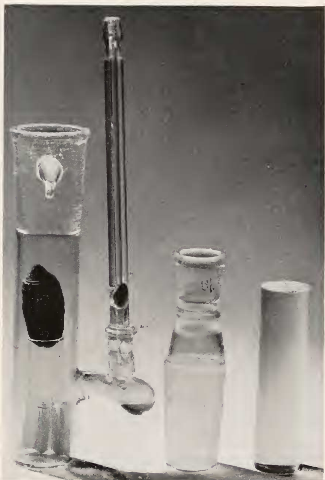
FIGURE 1. Respirometer vessel for use with standard Warburg manometer. The vessel is equipped with a side-arm, a venting-plug, and an adapter for junction with the manometer. The pupa is supported on a glass tube above alkali-moistened filter paper. The lucite cylinder on the extreme right is a space occupier for increasing the sensitivity of the system.
